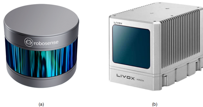
Figure 5. LIDAR: (a) Mechanical Scanning LIDAR, (b) Solid-state LIDAR.
